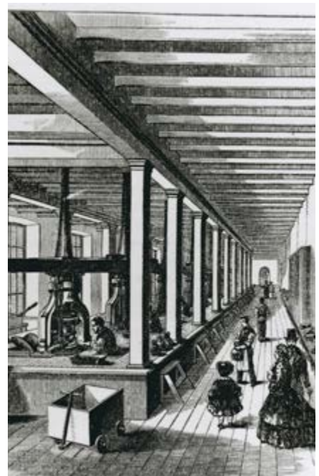
The coining press room at Tower Hill, equipped with Matthew Boulton's steam-powered presses, contrasted sharply with the arrangements in the Tower
