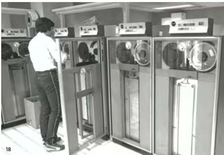
18. 1968, Computing centre: The electronic data storage devices are prepared at the SPARDAT computing centre that contain the journal entries for same-day entry and are sent to all branches in the country through the SPARDAT electronic network. Photo credit: Erste Group Bank AG, Corporate Archives
