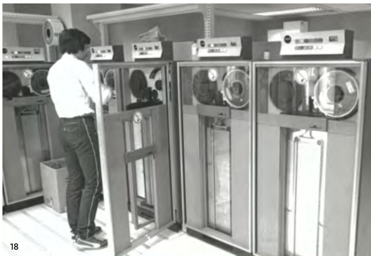
18. 1968, Computing centre: The electronic data storage devices are prepared at the SPARDAT computing centre that contain the journal entries for same-day entry and are sent to all branches in the country through the SPARDAT electronic network. Photo credit: Erste Group Bank AG, Corporate Archives
